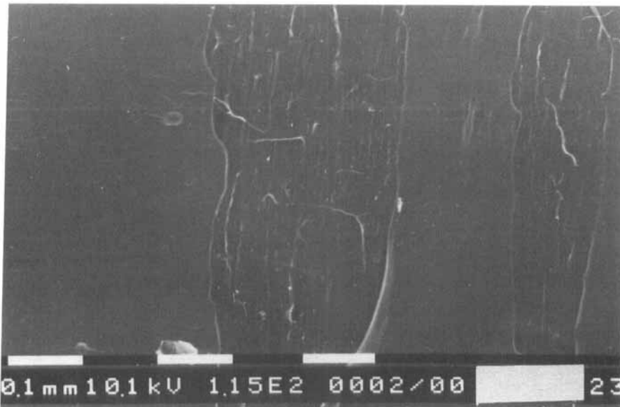
FIGURE 15 PP surface of laminate “B,” bond tested at 23°C.
